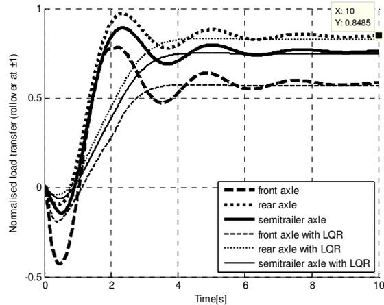
Fig3. Lateral load transfer with a LQR controller
