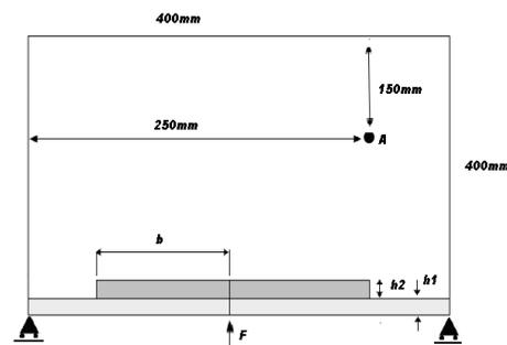
Fig1.. Rectangular acoustic cabin with two close pins
