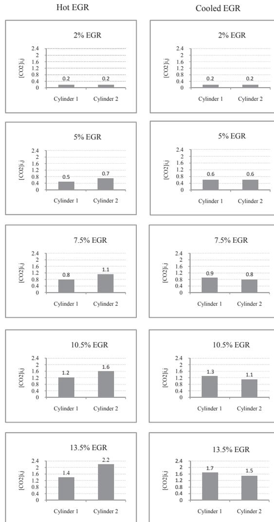
Fig. 12. CO<sub>2</sub> concentration at each inlet port in cases of hot and cooled EGR for various EGR rates at 1900 rpm engine speed, 100% load.
