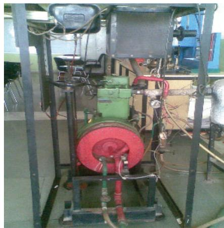
Plate 2. Rope Brake Dynamometer
