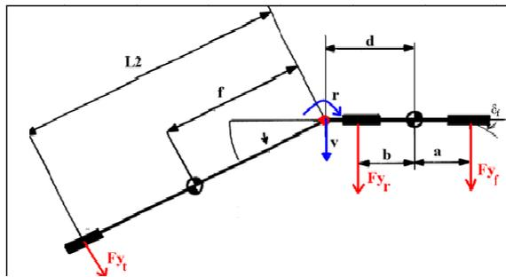
Fig. 5. Linear Model of Articulated vehicle [10]
