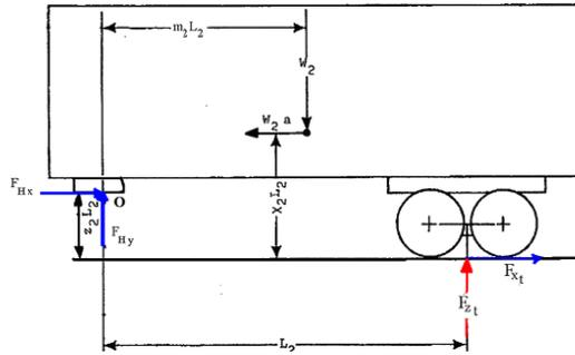
Fig. 2. Dynamic model of the trailer unit [7]
