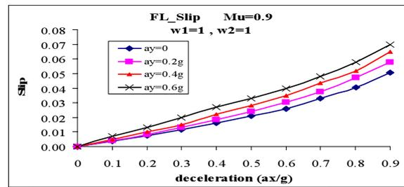
Fig. 6. Desired slip value for front left wheel
