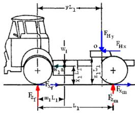
Fig. 1. Dynamic model of the tractor unit [7]
