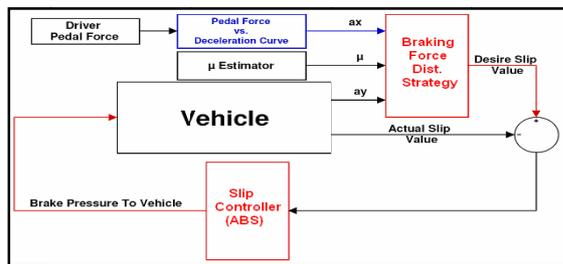
Fig. 8. Block diagram of the proposed EBD system
