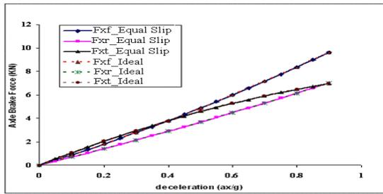
Fig. 4. Comparison of classical brake distribution and equal slips distribution
