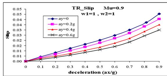
Fig. 7. Desired slip value for trailer right wheel
